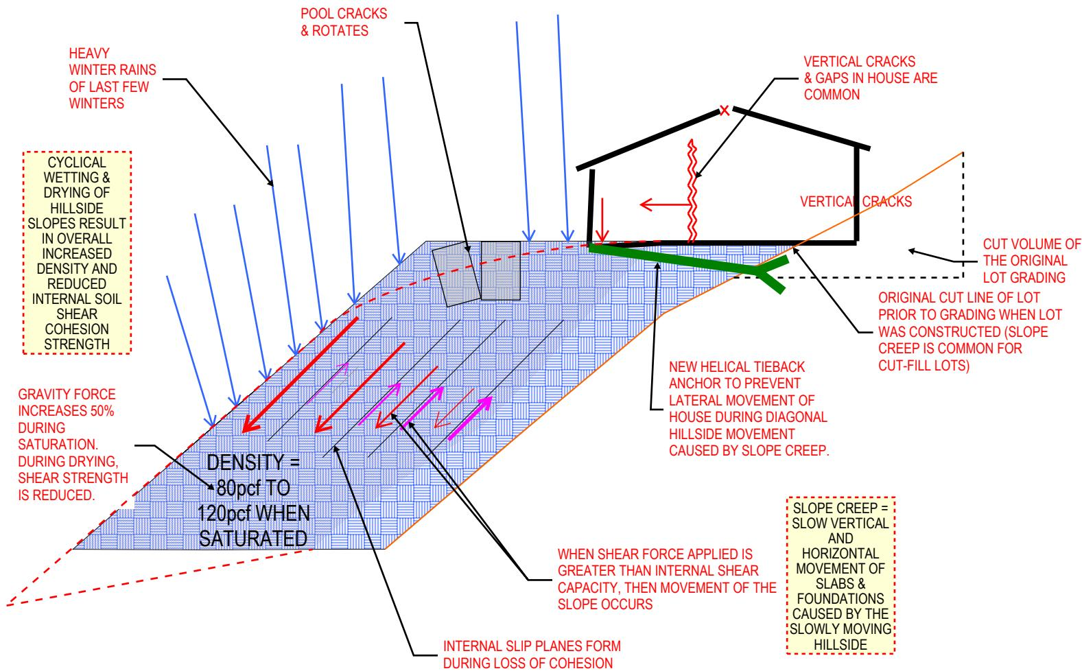
The homeowner should guard against slope creep by considering the probable explanations of causes of slope creep from a geologist or geotechnical engineer, which may include:
