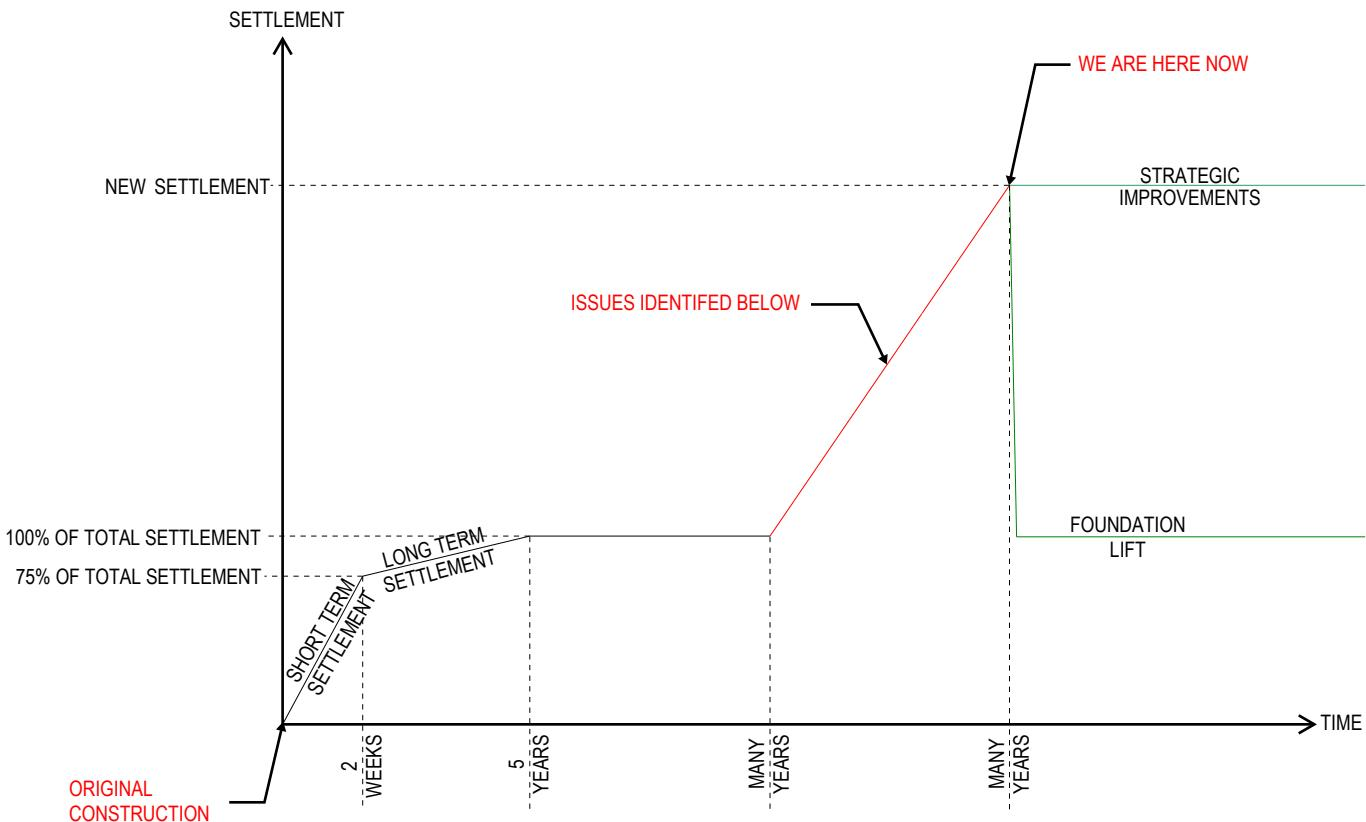
Differential settlement occurs when soil under a footing compresses, consolidates, or moves. The cause of soil compression or consolidation could be either:
