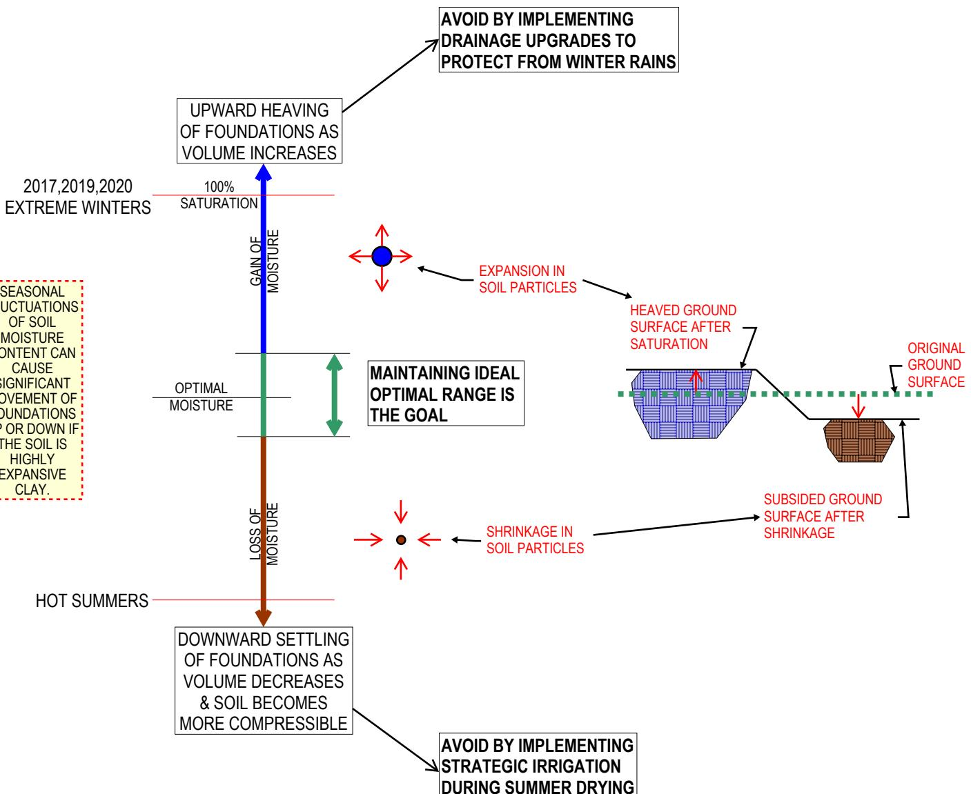
b) Clayey soils have a high expansion and contraction rate. Upon moistening, these soils expand. This diagram is for soil not loaded from the top with gravity forces such as the weight of the house. See next diagram for that.
