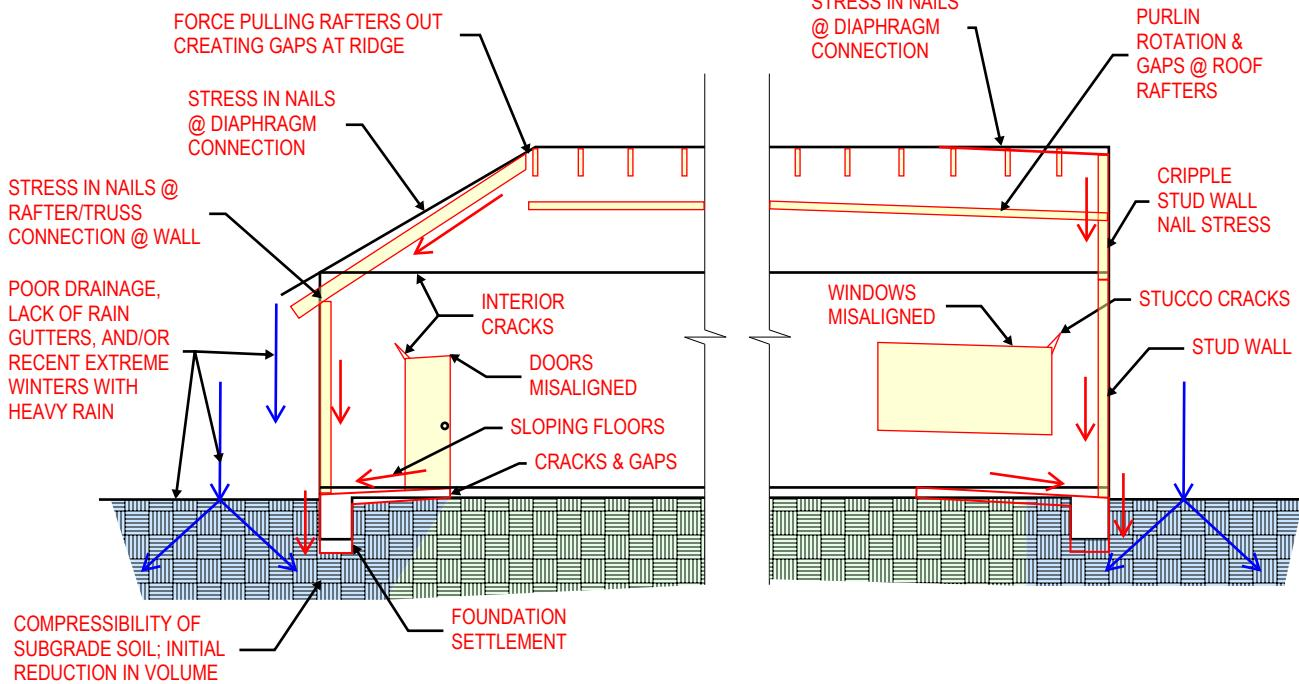
The level of stress in the connections and members of the structural framing system depends on the induced displacement caused by settlement.
