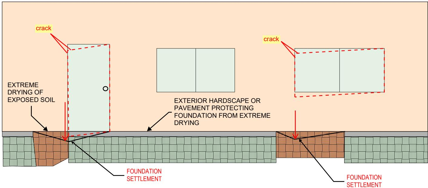
Gravity forces push the mass of the house down. The previously over-saturated soil consolidates (and shrinks if clay) is permanent and irrecoverable as the air voids between particles are eliminated. The foundation is permanently displaced downward and never recovers even if clay soil is saturated again.
